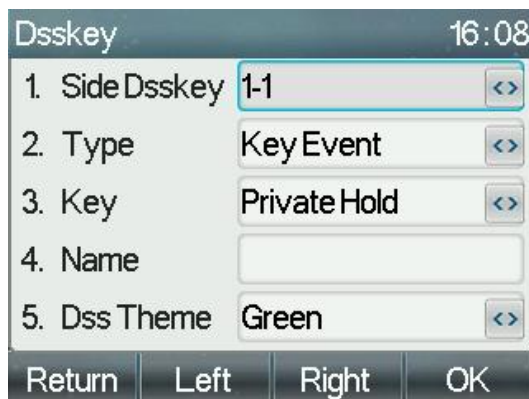
Picture 103 - DSS LCD key Page Configuration Screen
